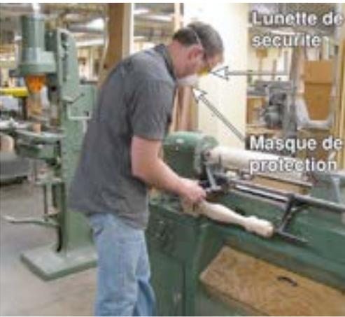
A photograph showing a worker in a grey t-shirt and blue jeans operating a green lathe. The worker is wearing safety glasses and a face mask. Labels with arrows point to the worker's eyes, labeled 'Lunette de sécurité', and the face mask, labeled 'Masque de protection'. The lathe is in a workshop setting. |
