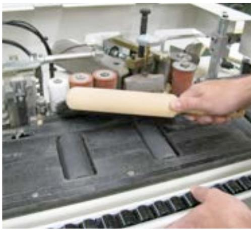
A close-up photograph showing a person's hands using a long-handled brush to clean a dark, industrial machine. The machine has several orange-colored rollers or spindles. The person is holding the brush horizontally, sweeping it across the machine's surface. The background is slightly blurred, showing more of the machine's structure. |
