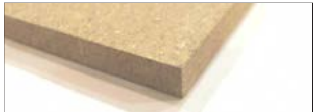
Figure C1.3.5 Panneau de fibres
