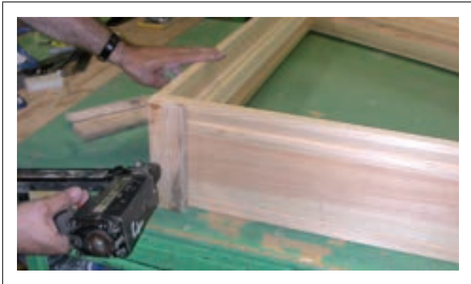
Figure C9.3.27 Clouage de lattes (talons)
