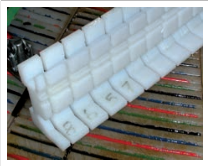
Figure C8.2.25 Installation du gabarit de pliage
