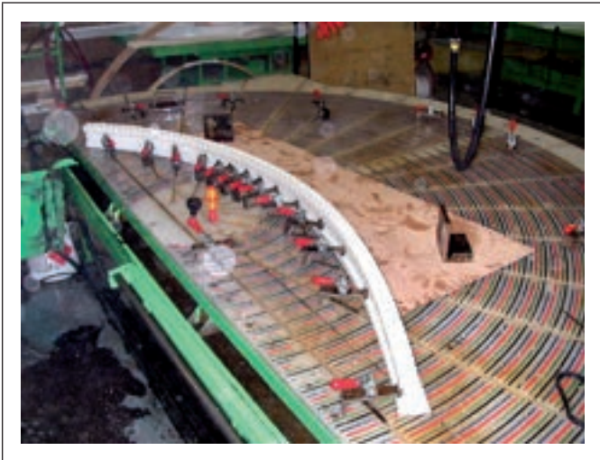
Figure C8.2.25 Installation du gabarit de pliage
